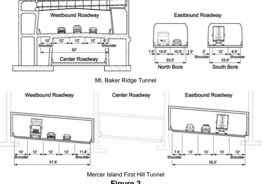
Figure 2 Existing I-90 Tunnel 3-Lane Cross-Sections (Typical)
