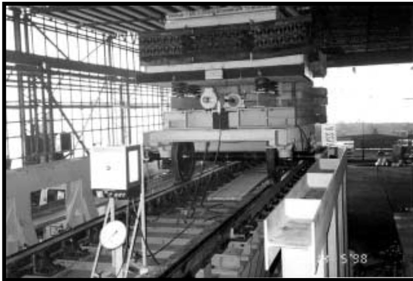
Photo #5 - Dynamic testing of Expansion Joint at Shop
