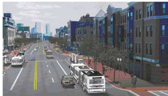
Arterial portion of the Silver Line uses curb-side lanes with significant improvements to the sidewalks and curbs to accommodate the stations.
