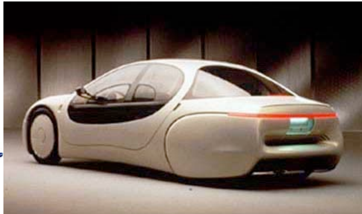
GM Composite Car built by Scaled Composites, 420 lb body
