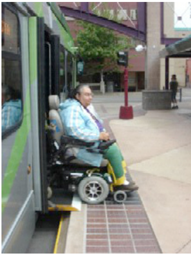
Figure 15 Wheelchair Customer Using Ramp to Board EmX
